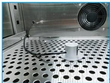
High water-proof grade illumination sensor
